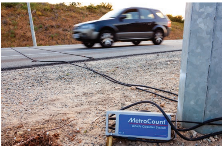
The RoadPod VT can classify any type of vehicle according to standard or custom class schemes from around the world.
