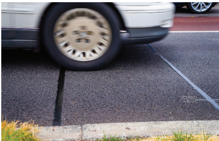
Piezoelectric sensors are highly sensitive, low-profile, durable and can withstand snow clearing.
