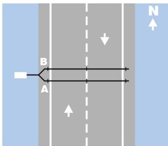
When installing one unit across two lanes of bidirectional traffic, careful consideration must be paid to the level of data quality degradation. Since sensors are placed parallel to each other, issues appear when two vehicles traverse them simultaneously. The sequence of axle hits produced by such an event makes it difficult to discern actual vehicles.
