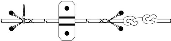
6. Attach Figure-8 cleats to the kerb side of each tube, using two per tube, and secure to the road using road nails or screws.
