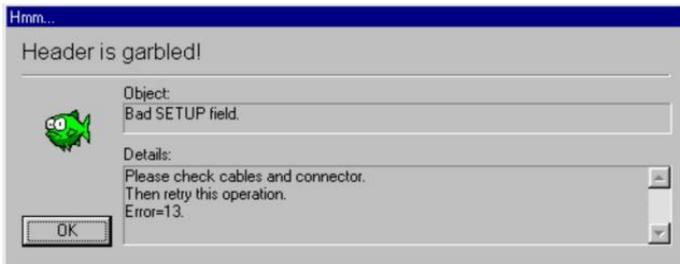
If you encounter this message, you will need to perform a Factory Setup operation in MTE. This will reset the unit and switch it to Active Logging state.
