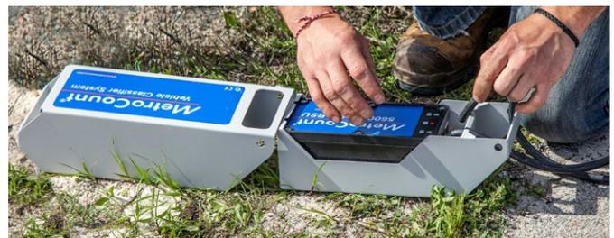
13. Slide the tray into the outer case and secure the counter using a padlock through one of the handle holes.
