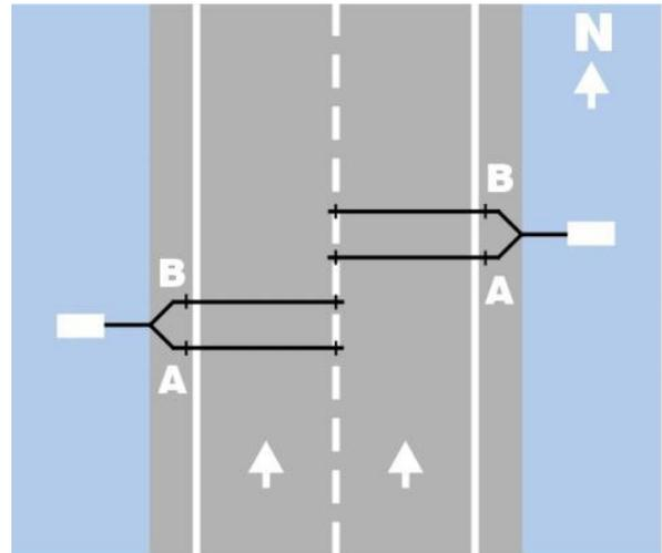
A two-lane road with a central median requires two RoadPod's to properly monitor both lanes.
