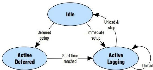
The *Idle* state is the unit's standby mode, meaning the counter does not log any data and simply retains the existing data.
