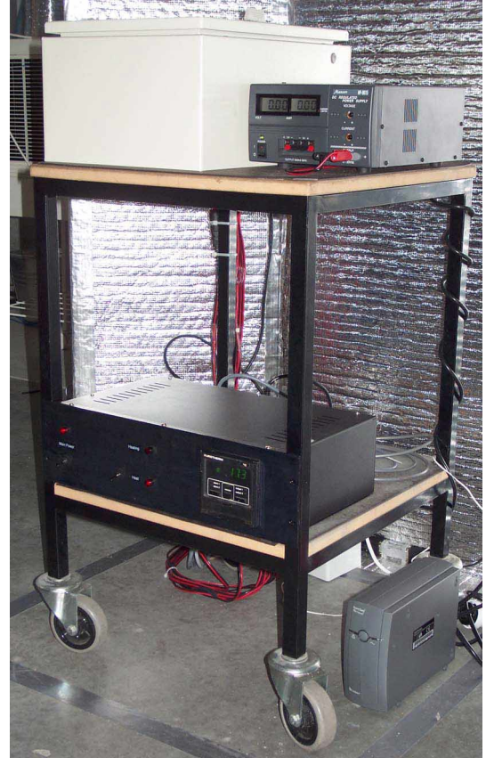
Custom-built oven for heating cycle, and controlling hardware.
