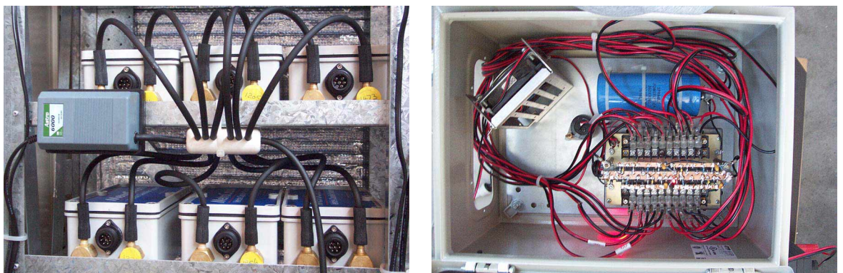
Custom pulse generator connected to tuned manifold, and driving circuitry.
